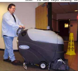
With a push of a button and a no-tools hose change, the operator moves from hard-surface floor scrubbing to carpet extraction with the Advance Adphibian
